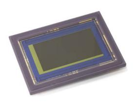
The 35MMFHDXS CMOS sensor delivers high-sensitivity, low-noise imaging performance, even in exceptionally low-light environments. The sensor's pixels and readout circuitry employ new technologies that reduce noise, which tends to increase as pixel size increases. High sensitivity and increased well depth have been achieved through a larger pixel size of  $19\mu m \times 19\mu m$  (square) with proprietary device design technologies. The 35MMFHDXS CMOS sensor is available in RGB or Monochrome.
