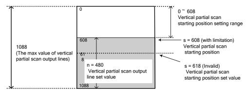
\* At manual partial scan mode, manual shutter value to be set shall meet the following conditions.
