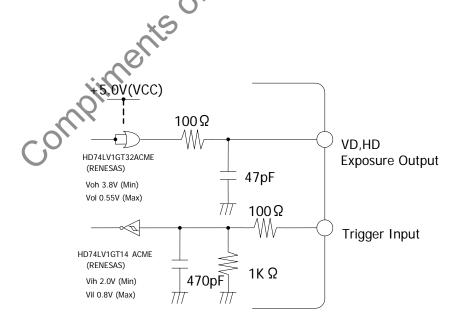
6pins Circular Connector at rear: GPIO interface
