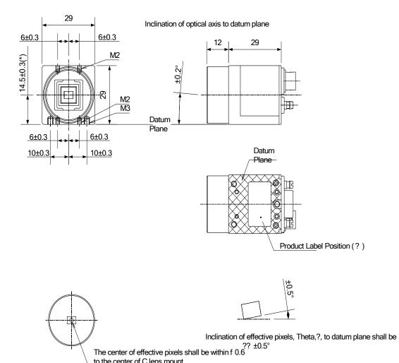
(\*) Dimensions from datum plane to the center of the lens mount
