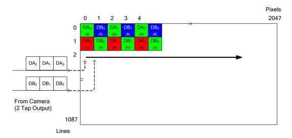
\* At manual partial scan mode, Bayer Pattern changes per 1 line according to the set vertical starting position value.
