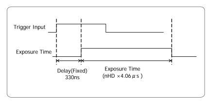
XVideo output signal delays by 2H from Exposure Time.
