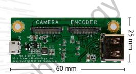
The CIB-HDMI-01 is designed to enable HDMI splitting for Sony 4K and HDMI cameras. The CIB-HDMI-01 takes the raw camera feed through the Camera KEL connector and uses the Second KEL connector to feed the encoder to provide a compressed output. The HDMI 1.4a is a no latency pass-through directly from the Camera.
